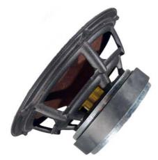
The basket is made of magnesium giving several benefits: First of all it makes it possible to create a very open basket – even behind the spider – thus ensuring high airflow at low frequencies, avoiding reflections at high frequencies and preventing under-/overpressure causing mechanical losses.
